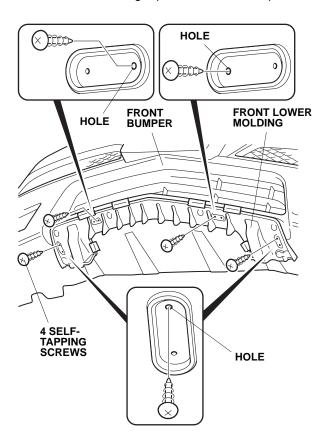
6. Push and check the outside edge of the front lower molding to make sure there is no gapping.
