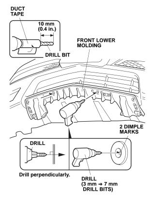
8. While wearing eye protection, drill a hole through the center of the two dimple marks. First drill with a 3 mm drill bit, and finish with a 7 mm drill bit. Remove any burrs from the edges of the holes with a file.
