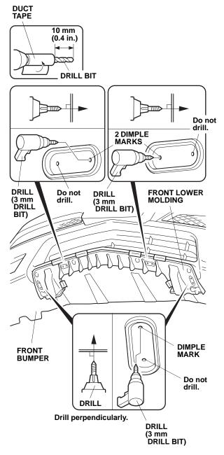
4. While wearing eye protection and holding the front lower molding against the front bumper, drill a hole through the center of the four dimple marks. Drill with a 3 mm drill bit. Remove any burrs from the edges of the holes with a file.
