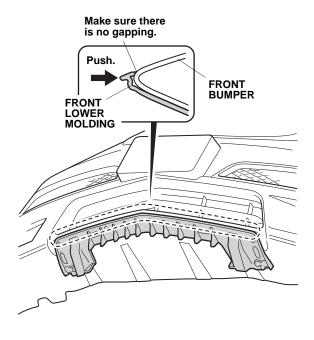
NOTE: If a gap is found to the outside edge of the front lower molding, remove the self-tapping screws, and realign the front lower molding. Repeat steps 3 and 4 to drill on the four alternate locations, and then reinstall the self-tapping screws to the alternate locations.
