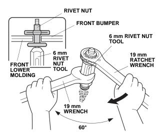
17. Remove the 6 mm rivet nut tool from the rivet nut by turning 6 mm rivet nut tool body in a counterclockwise direction.
