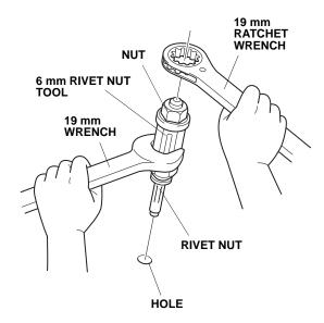
16. Turn the 19 mm ratchet wrench clockwise while holding the 6 mm rivet nut tool perpendicular to the work. Turn the nut until firm resistance is felt. Several turns will be required.
