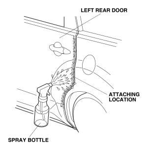
16. Open the left rear door again. Peel back about 50 mm (2 in.) of adhesive backing from the left rear door edge film. Align the V-notch in the door edge film with the end of the character line on the upper part of the left rear door.
