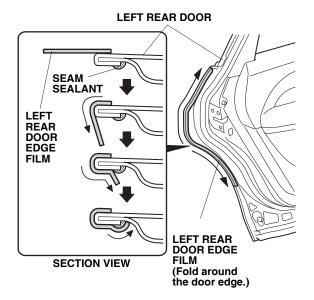
21. Using a lint-free shop towel, wipe up any excess water from the door edge film. Allow the door edge film to dry thoroughly.
