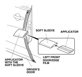
When you are satisfied that the door edge film is firmly attached to the edge of the driver's door, slowly remove the outer protective film.
