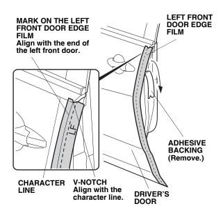
4. Continue to remove the adhesive backing while you align the mark on the left front door edge film with the end of the driver's door. Go to step 9.
