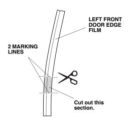
Partially peel back the adhesive backing from the upper part of left front door edge film. Align the V-notch in the upper part of door edge film with the end of the character line of the driver's door.
