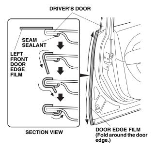
12. Using a lint-free shop towel, wipe up any excess water from the door edge film. Allow the door edge film to dry thoroughly.
