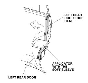
19. When you are satisfied that the left rear door edge film is firmly attached to the edge of the left rear door, slowly remove the outer protective film.
