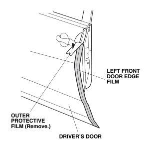
11. Starting in the middle of the door edge film and working outward, fold the door edge film around the edge of the driver's door using your fingers. Move your fingers in one direction. Attach the door edge film over the seam sealant. Do not trim or damage the seam sealant.
