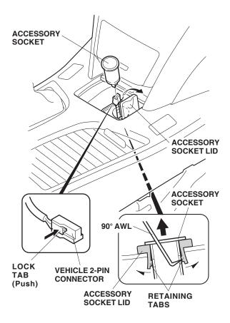
7. Push the lock tab in and disconnect the vehicle 2-pin connector from the accessory socket.
