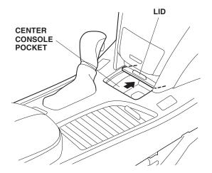
Open the accessory socket lid. Remove the accessory socket by reaching in from the driver's console trim opening and pushing up on the accessory socket. Use a 90° awl to release the two retaining tabs.
