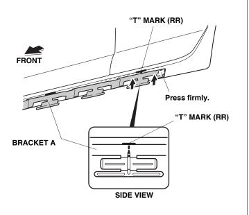
10. Temporarily detach the front end of side lower bracket where you lightly pressed in step 8. Keep holding the end of the bracket. Position the top of the bracket to the "T" mark (FR), and press on the front of the bracket firmly to adhere.
