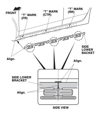
8. Raise the front of the side lower bracket to contact the "T" mark (FR). Press on the front of the bracket (where you removed the adhesive backing) lightly to adhere.
