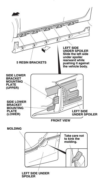
17. Pull the left side under spoiler lightly toward you and check that all the five resin brackets fit on the side lower bracket mounting plates securely. Visually check that the left side under spoiler is installed securely. If it is loose, repeat the installation procedure.
