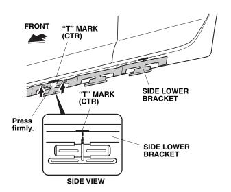
12. Check that the side lower bracket is in contact with the marks. Remove the two adhesive backings from the side lower bracket, starting at the center and working outward while lightly pressing on the bracket.
