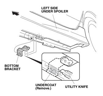
21. Install the bottom bracket in the position shown using two screws.
