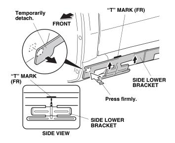
11. Position the top of the side lower bracket to contact the "T" mark (CTR), and press on the bracket to firmly adhere.
