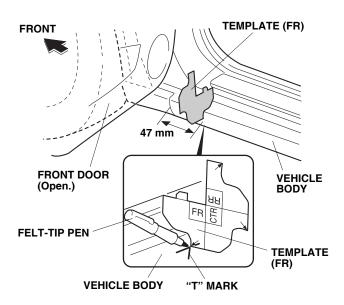
2. Position the template (marked CTR) on the vehicle body. Using a felt-tip pen, mark the vehicle body at the measurement shown.
