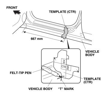
3. Open the left rear door. Position the template (marked RR) on the vehicle body. Using a felt-tip pen, mark the vehicle body at the measurement shown.
