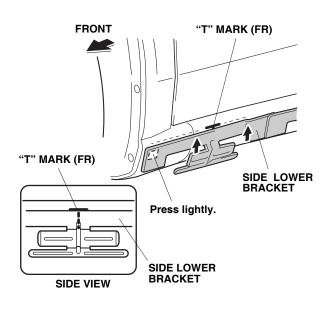
9. Raise the rear of the side lower bracket to contact the "T" mark (RR). Press on the rear of the bracket (where you removed the adhesive backing) firmly to adhere.
