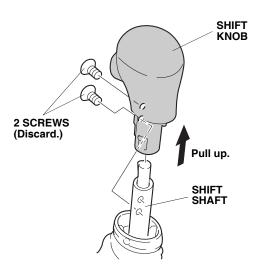
Install the select knob using the two new screws. Using a TORX screwdriver, torque the screws to 1.57 N·m (14 lb-in) Do not overtighten the screws.
