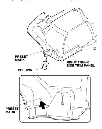
6. While wearing eye protection, drill the pierced mark to 6.5 mm. First drill with a 3 mm drill bit and finish with a 6.5 mm drill bit.
