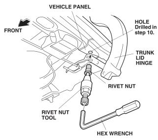
While holding the tool with the hex wrench, use a 19 mm wrench to turn the tool in a counterclockwise direction until the rivet nut is fully collapsed.
