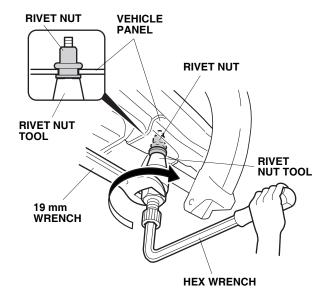
Remove the tool from the rivet nut by turning the hex wrench clockwise. 13. Reinstall the right trunk side trim panel, and install an anchor to the 6 x 20 mm flange bolt. Turn the "T" anchor in the direction shown.
