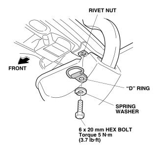
15. Remove the left trunk side trim panel, and repeat steps 5 through 13 to install a "T" anchor and a "D" ring on the left side of the vehicle.
