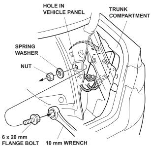
Locate the hole in the vehicle panel. Install one 6 x 20 mm flange bolt through the vehicle panel hole, then install a spring washer. Reinstall the stereo amplifier and a nut, and tighten. Be careful not to drop the bolt. 10. In the rear metal shelf, locate the hole near the trunk hinge arm.
