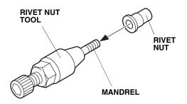
• Insert the rivet nut into the hole you just drilled, and install the hex wrench to the rivet nut tool.
