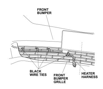
26. Attach the protective cap to the front bumper grille, and plug the connector of the heater harness into the protective cap.
