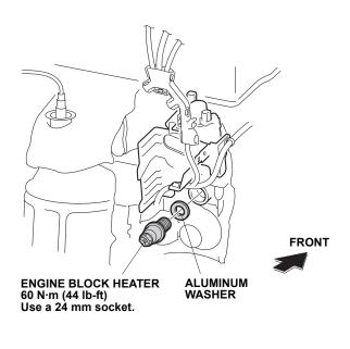
17. Plug the connector end of the heater harness into the engine block heater. Route the heater harness as shown, and secure the two wire ties with clip (points A and B) to the vehicle bracket.
