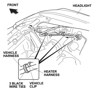
23. Route the heater harness as shown, and secure the wire tie with clip (points G) to the vehicle frame.
