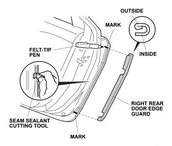
13. Position the cutting edge of the seam sealant cutting tool against the door edge, and trim the seam sealant from mark to mark between the marks at the top and bottom of the door edge.
