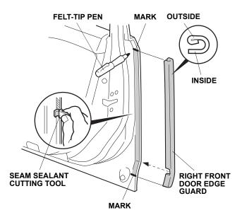
5. Position the cutting edge of the seam sealant cutting tool against the door edge, and trim the seam sealant from mark to mark between the marks at the top and bottom of the door edge.
