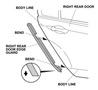
Using a felt-tip pen, mark the inside edge of the rear door at the upper and lower ends of the right rear door edge guard.
