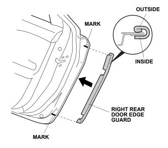
16. Using a rubber mallet, lightly tap around each bend in the right rear door edge guard.
