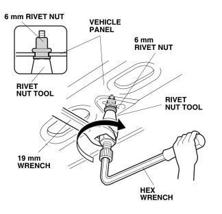
4. Remove the rivet nut tool from the 6 mm rivet nut by turning the hex wrench clockwise.
