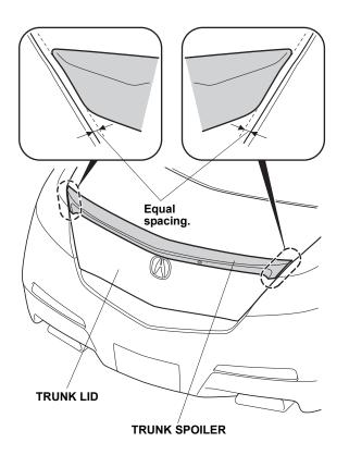
17. Install the trunk spoiler on the trunk lid using the three pins. Install the pins securely by applying pressure on the trunk spoiler with the palm of your hand.
