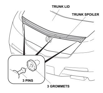
18. Open the trunk lid, and check that three pins are seated properly in each grommet.
