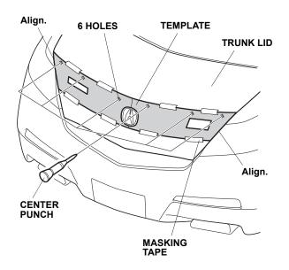
6. Center-punch the trunk lid at the six holes in the template. Remove the template.
