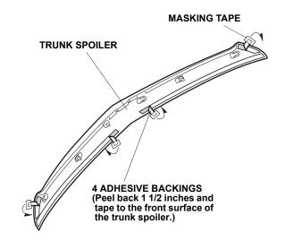
10. Using the alcohol pads, clean the trunk lid where the trunk spoiler will attach. Allow the alcohol to dry.
