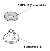
12. Install the three grommets to the trunk lid in the holes shown.
