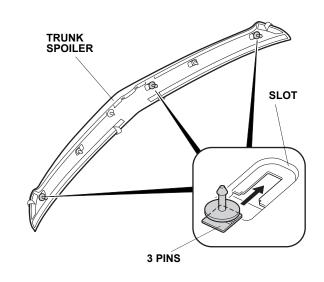
14. Install three seals (1 mm thick) to each of three pins.
