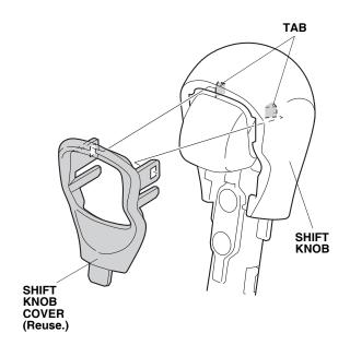
4. Remove and discard the two screws from shift knob, and remove the shift knob by pulling it up.
