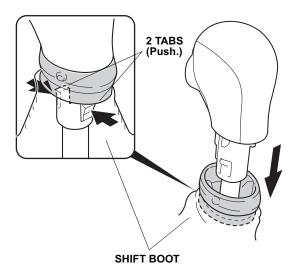
3. Pry out from the bottom of the shift knob cover and remove the cover.
