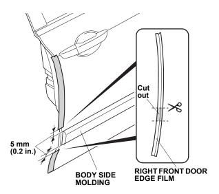
6. Continue to remove the adhesive backing while you align the centerline on the door edge film with the edge of the door.
