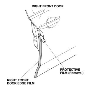
Starting in the middle of the door edge film and working outward, fold the door edge film around the door edge using your fingers. Move you finger in one direction. Attach the film over the seam sealant. Do not trim or damage the seam sealant.
