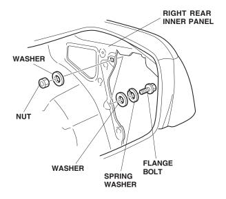
Reinstall all removed parts. Check that all clips are installed securely. 9. Install the anchor to the flange bolt.
