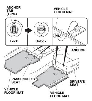
2. Position the driver's and passenger's all season mats by aligning the tabs with their anchors.
