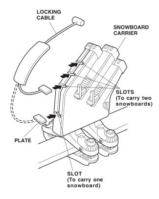
15. After loading the snowboards on the carrier, adjust them with the help of the board supports so that the top edges are level and the boards are as far down in the carrier as possible. To secure the snowboards, use the key to open the covers, and insert the locking cable stoppers into the holes in the carrier covers.
