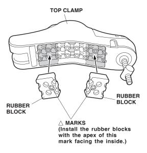
△ MARKS (Install the rubber blocks with the apex of this mark facing the inside.)
