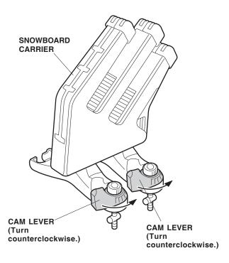
Attach the two bottom clamps to the two top clamps.
