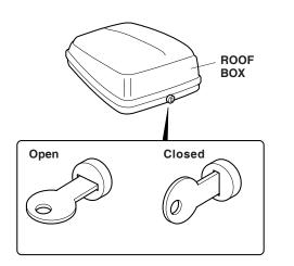
**Locking:** Press down on the lid. There should be an audible click. Be sure the lid is latched by attempting to lift the lid. Turn the key clockwise to lock the roof box. Remove the key while not in use. Be sure the straps do not dangle from the roof.
