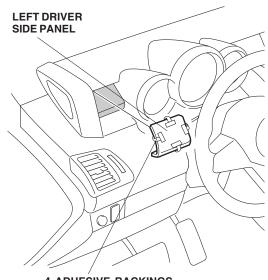
4 ADHESIVE BACKINGS (Press on the left driver side panel firmly while removing the adhesive backings.)
