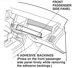
4. Press and hold the side panel for 30 seconds.
