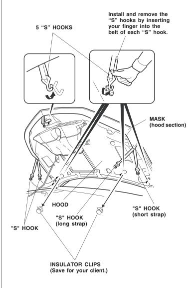
3. Fit the corners of the mask (hood section) around the hood. Adjust the mask so that it fits smoothly over the edges. Attach the two "S" hooks with the longer strap and red stitching to the inboard holes. Attach the two "S" hooks with the shorter strap to the outboard holes.
