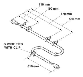
14. Plug the heater harness connector into the engine block heater.
