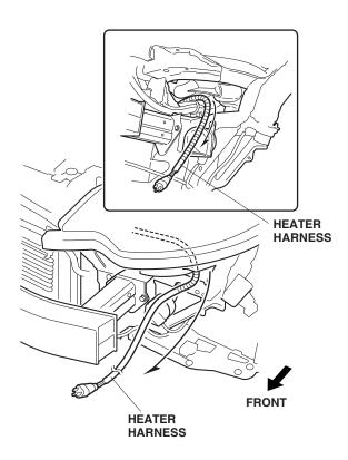
18. Secure the fifth wire tie with clip, which you installed on the heater harness, to the vehicle frame.
