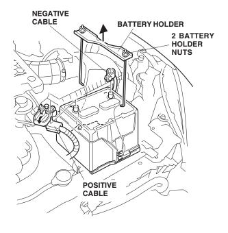
8. Remove the battery cover, battery and battery box.
