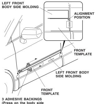
(Press on the body side molding firmly with the palm of your hand while removing the adhesive backings.)
