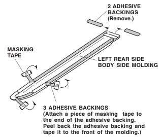
10. Align the front end of the left rear side molding with the rear template as shown, and temporarily attach it using the top end of the template as a guide.
