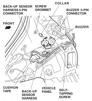
34. Plug the back-up sensor harness 5-pin connector into the buzzer 5-pin connector and secure the buzzer to the screw grommet with the self-tapping screw and collar. 35. Route the back-up sensor harness up along the vehicle harness, and secure it to the vehicle harness with five wire ties. Don't secure the back-up sensor harness to the SRS harness.
