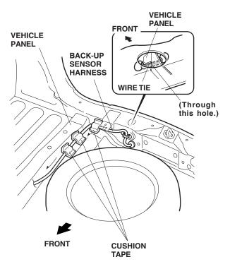
28. Route the back-up sensor harness forward and secure it to the vehicle panel with the two cushion tapes.
