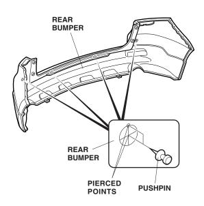
22. While wearing eye protection, drill a 3 mm pilot hole through each of the eight pierced points you just made from the outside surface of the rear bumper.
