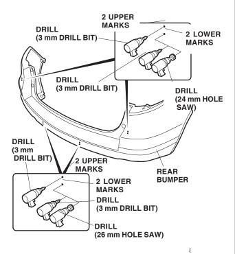
23. While wearing eye protection, enlarge the hole at each of the lower marks (center) using a 24 mm hole saw (outer holes) and a 26 mm hole saw (inner holes). Remove all burrs.
