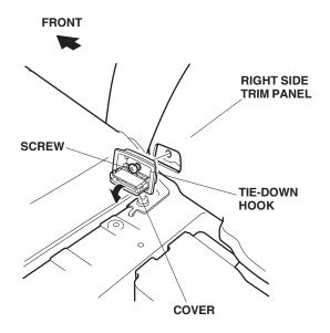
13. Open the right rear cover tie-down hook. Remove the rear tie-down hook from the right side trim panel (one screw).
