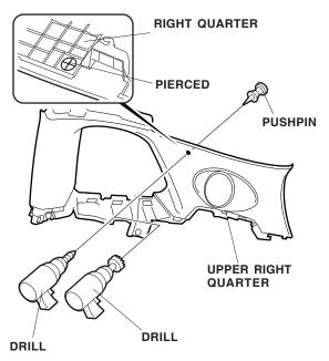
42. While wearing eye protection, drill a 19 mm hole at the pierced point from the outside surface of the right quarter pillar trim. Remove all burrs.
