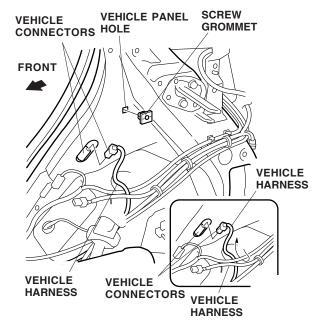
32. Disconnect the vehicle connector. Inside the vehicle panel, route the vehicle harness under the existing vehicle connector running along the fenderwell panel and reconnect the vehicle connector.
