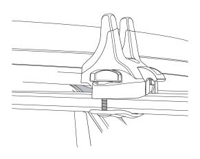
6. Slide the latch on one attachment strap into the clip on the base.
