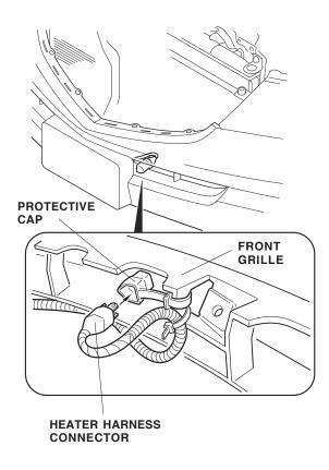
16. Secure the heater harness to the vehicle harness using four black wire ties.
