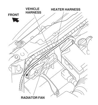
13. Route the heater harness along the vehicle harness and out the gap in the bulkhead frame as shown.
