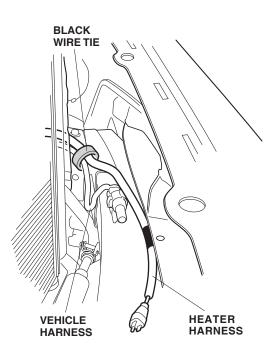
15. Using a black wire tie, secure the heater harness to the front grille as shown. Then attach the protective cap to the grille in the location shown, and install the heater harness connector into the protective cap.
