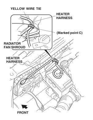
12. Route the heater harness to the left side of the radiator fan along the vehicle harness.
