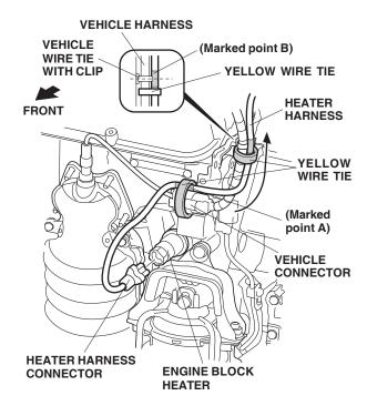
10. Secure the heater harness to the vehicle connector with one yellow wire tie at the marked point A. Secure the heater harness to the vehicle harness with one yellow wire tie at the marked point B. 11. Secure the heater harness to the radiator fan shroud with one yellow wire tie at the marked point C.
