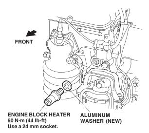
9. Route the heater harness down to the engine block heater. Connect the heater harness connector to the engine block heater.
