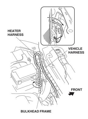
14. Secure the heater harness to the vehicle harness using one black wire tie.
