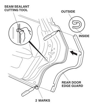
Position the cutting edge of the seam sealant cutting tool against the door edge and trim the seam sealant from mark to mark.
