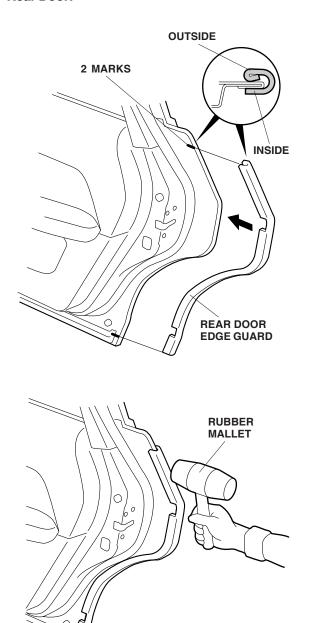
7. Repeat steps 1 through 6 to install the door edge guards on the other side of the vehicle.
