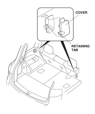
4. Install the cargo cover into the recess in the left rear side panel in the direction shown, then compress the cargo cover, and install it in the right rear side panel.
