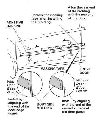
5. Position the molding on the door and align it with the masking tape. Remove the masking tape.
