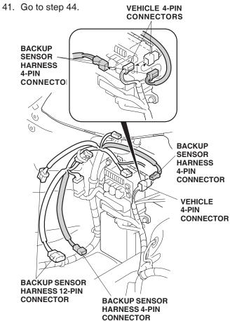
40. Plug the backup sensor harness 12-pin connectors into each other.
