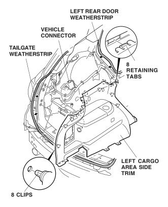
25. Remove the left cargo area side trim (eight clips, eight retaining tabs, and unplug the vehicle connector).
