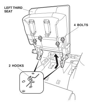
20. Release the two hooks by moving the left third seat rearward, then remove the left third seat.
