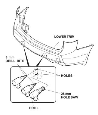
On the inside of the rear bumper, locate the two
