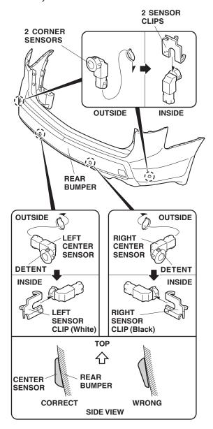
Install the right and left center sensors on the rear bumper using the right sensor (black) clip for the right sensor and the left sensor (white) clip for the left sensor.
