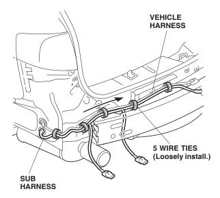
**Without Vehicle Harness:** Route the subharness along the bumper beam. Loosely install five wire ties with clips to the subharness and insert the clips into the five vehicle panel holes.
