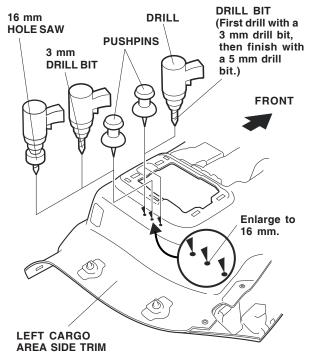
52. While wearing eye protection, drill a 3 mm hole through each of the three pierced points. Then drill the two outer holes with a 5 mm bit. Enlarge the center hole to 16 mm using a hole saw. Remove any burrs from the holes.
