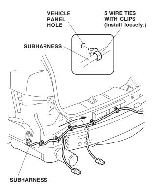
32. Install four clips to the subharness at the four thinner points on the subharness, then route the subharness along the rear bumper beam.
