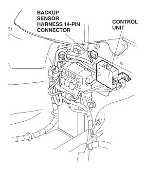
48. Using scissors, cut the EPT sealer as shown. Wrap the small piece of EPT sealer around the backup sensor 4-pin connector, and wrap the large piece of EPT sealer around the 12-pin connector.
