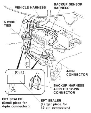
49. Secure the backup sensor harness to the vehicle harness using five wire ties.
