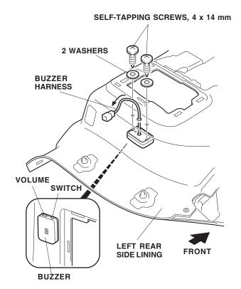
54. Connect the buzzer harness 2-pin connector to the backup sensor harness 2-pin connector. Secure the buzzer harness 2-pin connector to the vehicle harness using one wire tie.
