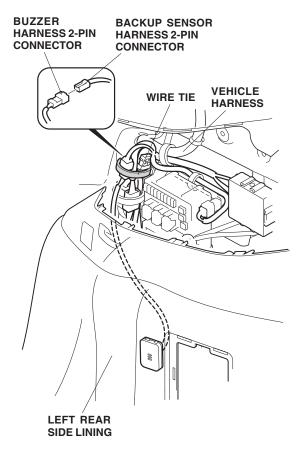
55. Plug in the vehicle connector, and reinstall the left cargo area side trim. Check that all clips and retaining tabs are installed securely.
