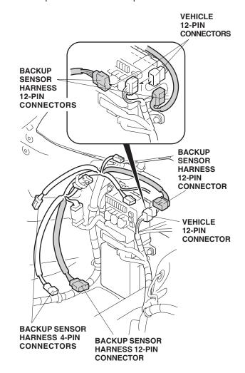
43. Plug the 4-pin connectors of the backup sensor into each other.
