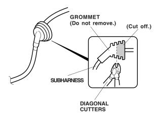
27. Locate and remove the body panel grommet from the left rear bumper area.
