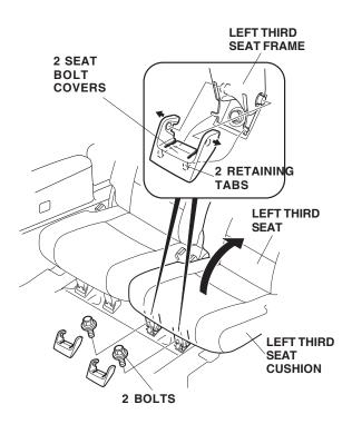
18. Remove the two bolts that fasten the left third seat to the floor. Raise the left third seat cushion.
