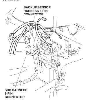
37. Remove the vehicle ground bolt from the ground terminal and attach the backup sensor harness ground terminal to the vehicle ground terminal using the vehicle ground bolt.
