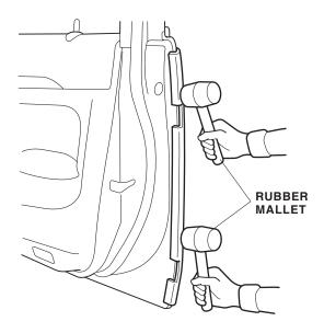
8. Repeat steps 3 thru 7 to install the left front door edge guard.
