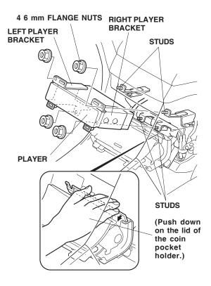
20. Insert two player panel hooks into the square holes of the right and left player brackets, then insert two player panel clips into the latches.
