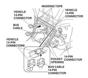
8. Wrap one wire tie with clip around the bus cable, and push the wire tie with clip into the hole in the vehicle frame.
