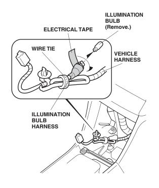
17. Apply masking tape as shown. Reinstall the coin pocket holder or ashtray holder.
