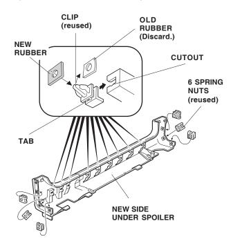
11. Install the six spring nuts removed in step 7 onto the front and rear ends of the new side under spoiler.
