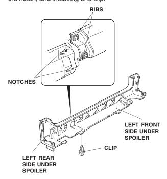
10. Slide the nine clips (removed in step 8) into the holders on the new side under spoiler through the slots, and align the tabs on the clips with the cutouts on the holders. Remove the existing rubber spacers from the clips, and install a new rubber spacer onto each of the nine clips.
