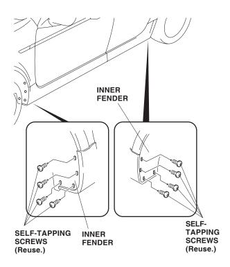
3. Remove the four self-tapping screws that fasten the rear inner fender to the fenderwell.
