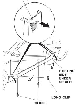
5. Pull the top of the spoiler out, at the front and rear ends, to release the three clips (one at the front and two at the rear).
