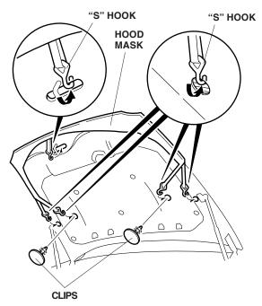
2. Fit the corners of the mask around the hood. Adjust the mask so that it fits smoothly over the edges. Attach the five "S" hooks to the hood.
