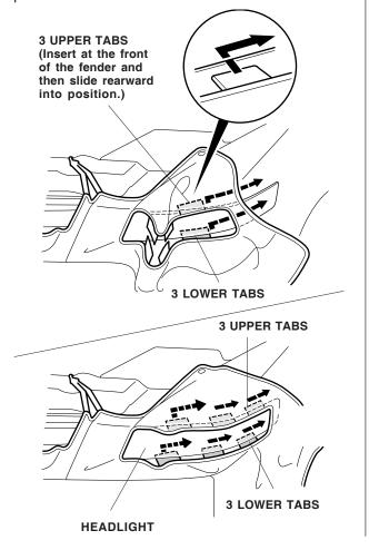
9. At the fender/bumper area, insert the small tab from the mask between the bumper and the fender.
