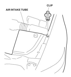
Install one new clip with a snap-screw into where you removed the clip, and tighten the snapscrew.
