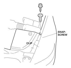
6. Pull the mask toward the left fender, and slip the left pocket of the bumper section onto the left front corner of the fender.
