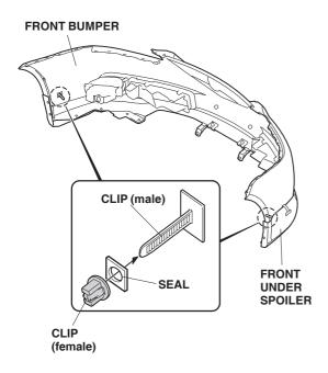
27. Secure the front under spoiler on the front bumper using two clips (female).
