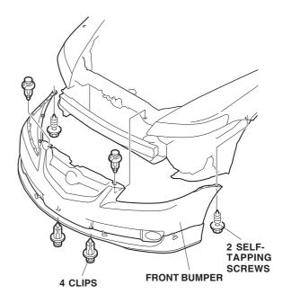
29. Secure the front bumper to the car using four clips, two clips (included in the kit) and two bolts.
