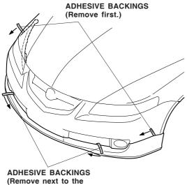
ADHESIVE BACKINGS (Remove next to the side adhesive backing.)
