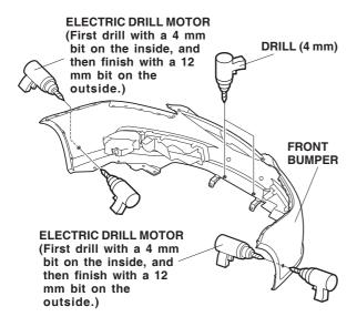
13. Position the left bracket on the inside of the front bumper. Mark the front bumper at the drill point. Align the top of the left bracket with the bead of the front bumper and align the recess at the rear of the left bracket with the flange of the front bumper.
