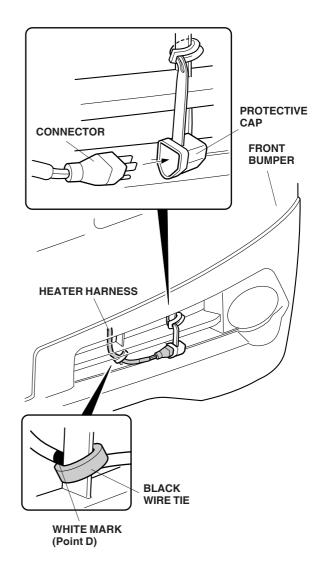
25. Attach the protective cap to the bumper grille, and plug the heater harness connector into the protective cap.
