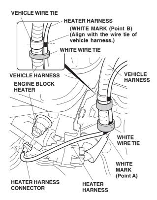
14. Align the white mark (point B) on the heater harness with the vehicle wire tie, and secure the heater harness to the vehicle harness with two white wire ties as shown.
