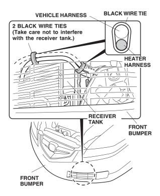
27. Secure the heater harness to the vehicle harness with two black wire ties.
