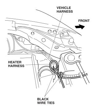
28. Secure the heater harness to the vehicle harness with three black wire ties as shown.
