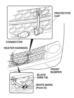
23. Attach the protective cap to the bumper grille, and plug the heater harness connector into the protective cap. Go to step 26.
