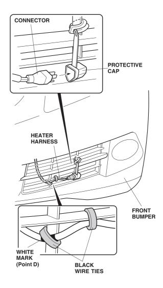
20. Attach the protective cap to the bumper grille, and plug the heater harness connector into the protective cap. Go to step 26.
