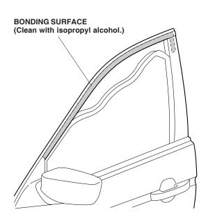
3. Attach a strip of the masking tape to the ends of the adhesive backings, and remove 50 mm to 80 mm (2 to 3 in.) from the ends. Fold back the ends and tape the ends to the front of the door visor. Note the direction of the adhesive backings.
