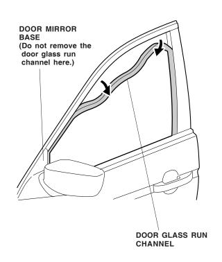
2. Using isopropyl alcohol on a shop towel, clean the shaded area of the door sash.
