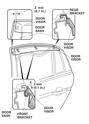
12. Adjust the location of the door visor so that the clearance between the door visor and door sash is 3 mm (0.1 in.) at the front end, and 3 mm (0.1 in.) at the top.
