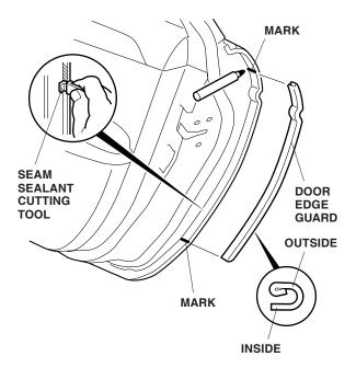
Position the cutting edge of the seam sealant cutting tool against the door edge and trim the seam sealant between the marks.
