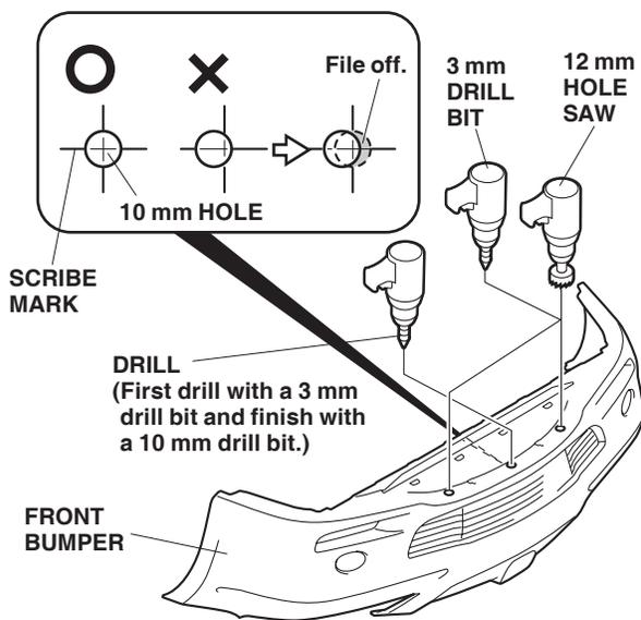
14. Mark the front bumper at the two points 10 mm inside from the two inner scribe marks out of the four marks that locate around the fog light opening in the front bumper. Pierce a pushpin through the marks you just made.
