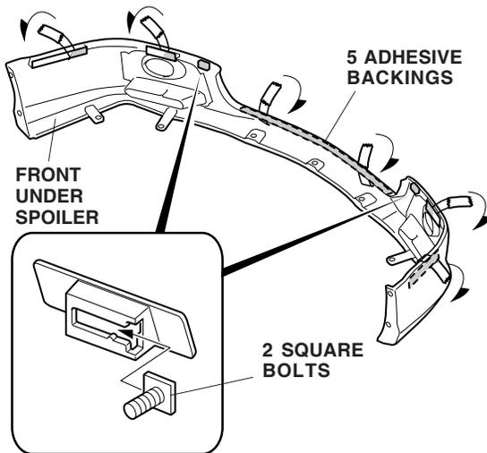
22. Using isopropyl alcohol on a shop towel, thoroughly clean the front bumper where the front under spoiler will attach.
