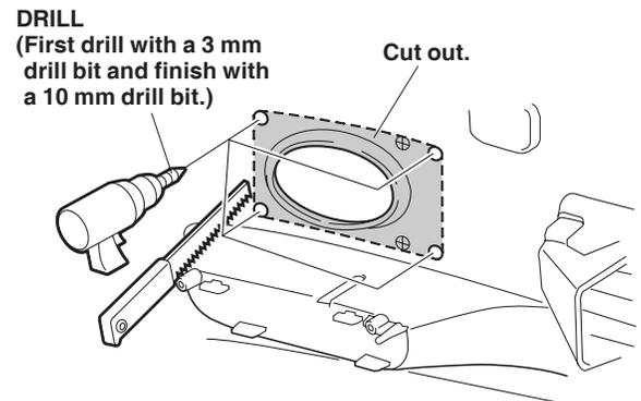
17. Draw the lines that pass the outer edge of each hole you just made. Cut out the front bumper along the lines, and remove the burrs from the edges of the hole.
