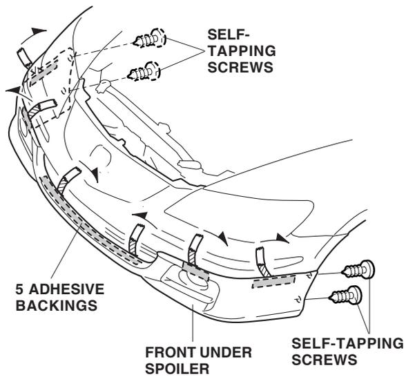
29. While holding light pressure on the spoiler, carefully remove the adhesive backings. Hold the spoiler firmly against the front bumper with the palm of your hand for 30 seconds.
