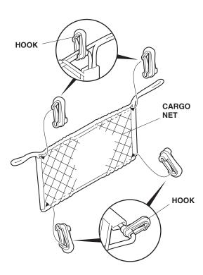
Install the cargo net to the tie down hooks and the anchors in the trunk. The cargo net can be installed in 2 different positions, vertically or horizontally.
