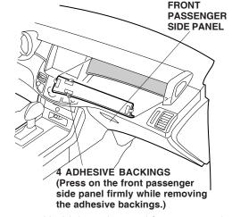
Press and hold the side panel for 30 seconds.
