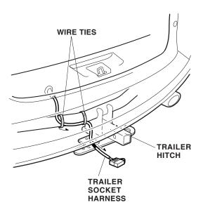
23. Attach the trailer socket harness 4-pin connector to the trailer hitch using the 6 x 16 mm flange bolt and the 6 mm flange nut.
