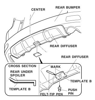
37. Using a pushpin, pierce the diffuser at both cross marks. Using a felt-tip pen, mark the outline of the template, then remove the template.
