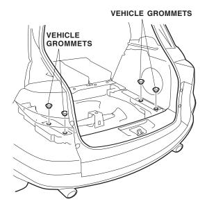
45. Insert the right and left plates into the holes exposed in the step 44.
