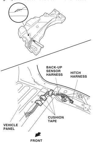
20. Plug the trailer hitch harness 4-pin connector into the trailer socket harness 4-pin connector.
