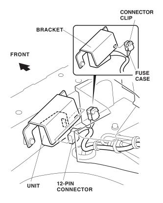
34. Rotate the control unit assembly down onto the right flange bolt. Torque both 6 x 20 mm flange bolts to 4.0 N·m (3.0 lb-ft)
