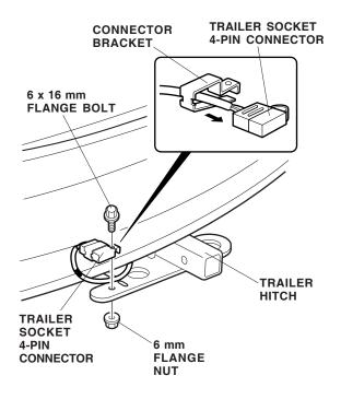
24. Secure the trailer hitch trailer socket harness to the trailer hitch at the green tape using one wire tie.
