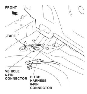
17. Near the 6-pin connector, secure the hitch harness to the vehicle harness with two wire ties.
