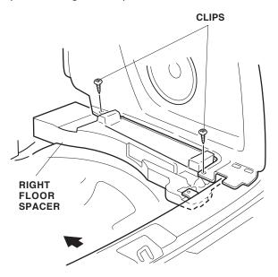
10. Remove the right floor spacer by gently pushing in at the back edge, and pulling out at the front edge to clear the vehicle bracket.
