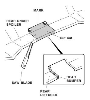
40. With the vehicle on a hoist, position template A on the rear bumper, and tape in place.
