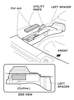
Locate the right spacer. Using a utility knife, cut out the right spacer in the area shown. Take care not to damage the vehicle harness under the right spacer.
