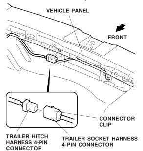
21. Secure the trailer socket harness 4-pin connectors to the vehicle panel using the connector clip.
