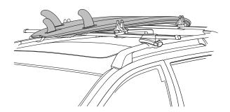
Adjust the position of the bases so that the bottom of the surfboard rests on the rubber part of the bases. Tighten all knobs firmly and evenly.
