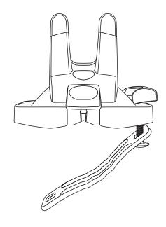
Position the base on the crossbar. Loosely install one bolt and knob as shown.
