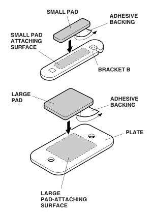
5. Using isopropyl alcohol on a shop towel, clean the four plates where the large pads will attach. Remove the adhesive backings from the large pads, and attach them to the plates. 6. Under the roof box, insert a bolt through bracket B, through the plate, and into the predrilled hole in the bottom of the roof box.
