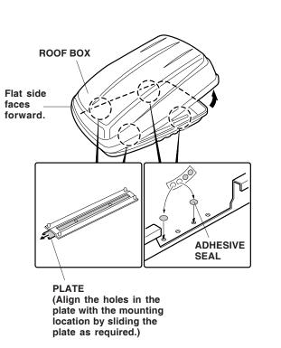
3. Attach an adhesive seal over each of the four unused mounting holes (two on each side) at the rear of the base of the box. The seals will help prevent water from entering the roof box.
