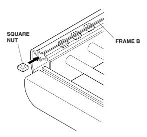
8. Position four bracket covers (A) over the ends of the frames A and B, then install four bracket covers (B) and install self-tapping screws to secure the cover.
