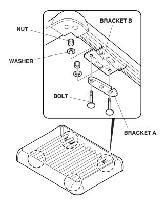
11. Position the roof basket on the roof rack, with the flap from frame A facing forward. Attach the basket to the cross bars by sliding bracket (A) around the crossbar and tightening the nuts. Make sure to tighten the nuts evenly.
