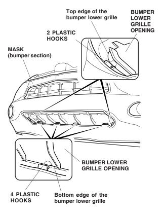
20. Attach the six plastic hooks to the bottom inside edge of the front bumper.
