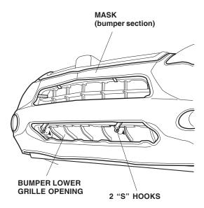
19. Attach the six plastic hooks to the bottom inside edge of the bumper lower grille opening.
