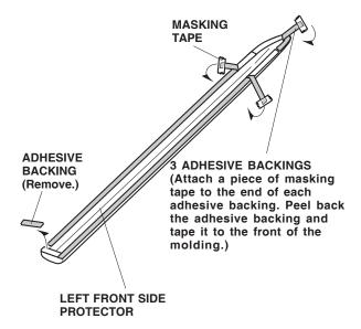
4. Align the rear end of the left front body side molding with the front template, and attach it using the top edge of the template as a guide.
