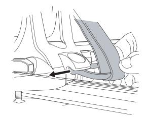
7. Rotate the latch up to lock it into the base. Repeat this step at the other base on the crossbar.
