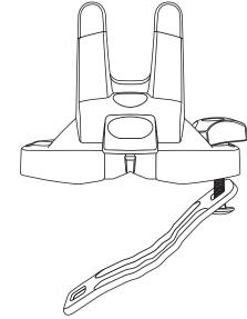
2. Position the base on one crossbar on the roof rack. Loosely install another bolt and knob as shown.
