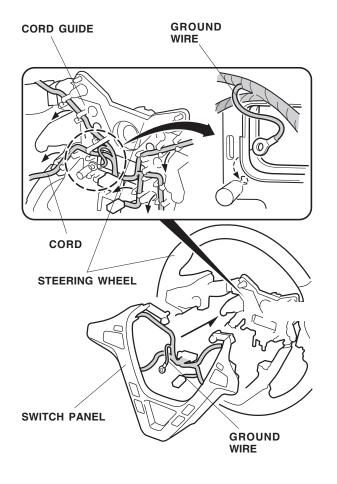
17. Install the steering wheel cover to the steering wheel with the eight self-tapping screws. Secure the ground wire with the self-tapping
