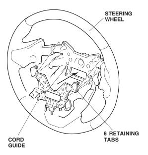
13. Position the switch panel to the steering wheel, and attach the cord to the retaining tabs on the steering wheel.
