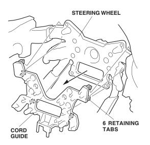
12. Install the cord guide on the new steering wheel.
