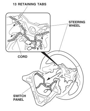
11. Pry up the six retaining tabs and remove the cord guide from the steering wheel.
