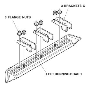
Loosely attach the Brackets C on the left running board to the Bracket A and Brackets B on the body with 12 short flange bolts and 12 flange nuts.
