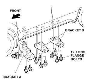
2. Remove the two pieces of paper holding the bolts on the bottom of the left running board.
