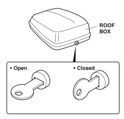
**Locking**: Press down on the lid. There should be an audible click. Be sure the lid is latched by attempting to lift the lid. Turn the key clockwise to lock the roof box. Remove the key while not in use. Be sure the straps are not outside of the roof box.
