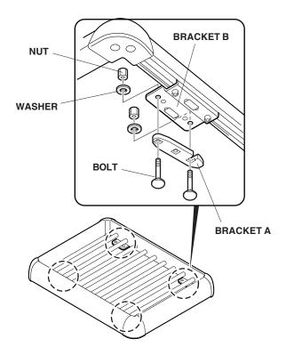
11. Position the luggage basket on the roof rack, with the flap at the front. Attach the basket to the crossbars by sliding bracket A around the crossbar and tightening nuts. Tighten the nuts evenly.
