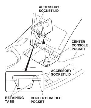
9. Slide the ring into the hole in the center console pocket in the direction shown.
